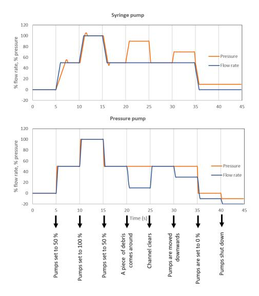
A side by side comparison (illustration) of syringe and pressure pump shows how the flow rates (as detected within a microfluidic chip) and pressures (as detected at the pump) react to different settings and situations. The behavior depends heavily on the settings — the illustration predicts a typical microfluidic chip with Essi pressure pump and Essi syringe pump with a glass syringe.
